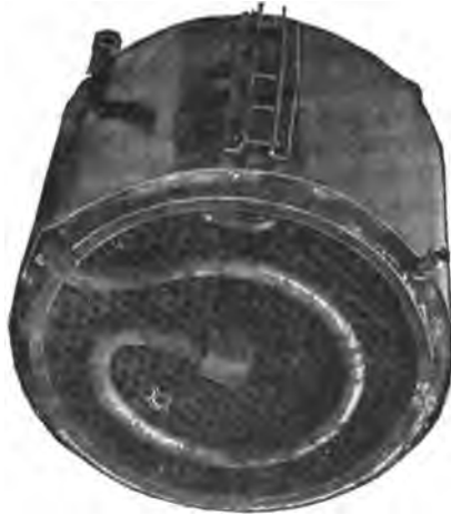
FIG. 149.--The Boiler used on the "Victor" Carriage, Bottom View, showing blow-off and steam superheating tube. In this boiler the steam connection is through a tube, about \frac{3}{8} inch below the upper tube plate, which passes down through the lower tube plate and is carried over the burner, as shown. The steam pipe then passes up through the lagging around the boiler and connects with the engine from the top.
